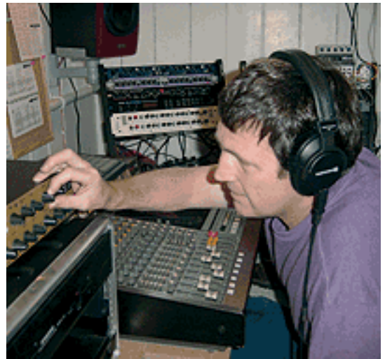
The SPL Channel One's Air EQ control was used to compensate for the high-frequency losses incurred because of the Tascam 388's worn heads.
