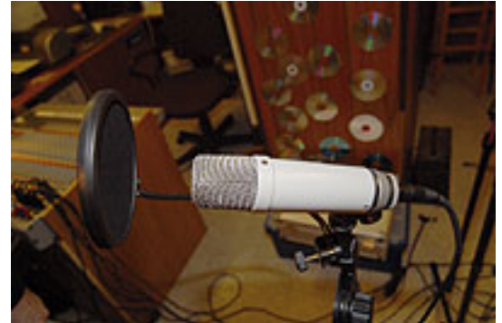
Paul and Hugh quickly noticed Peter's unusual vocal-miking setup! Given that the NT1 is a side-firing mic, a much clearer sound was immediately obtained by having the singer address the correct side of the mic, as marked with the gold dot.
