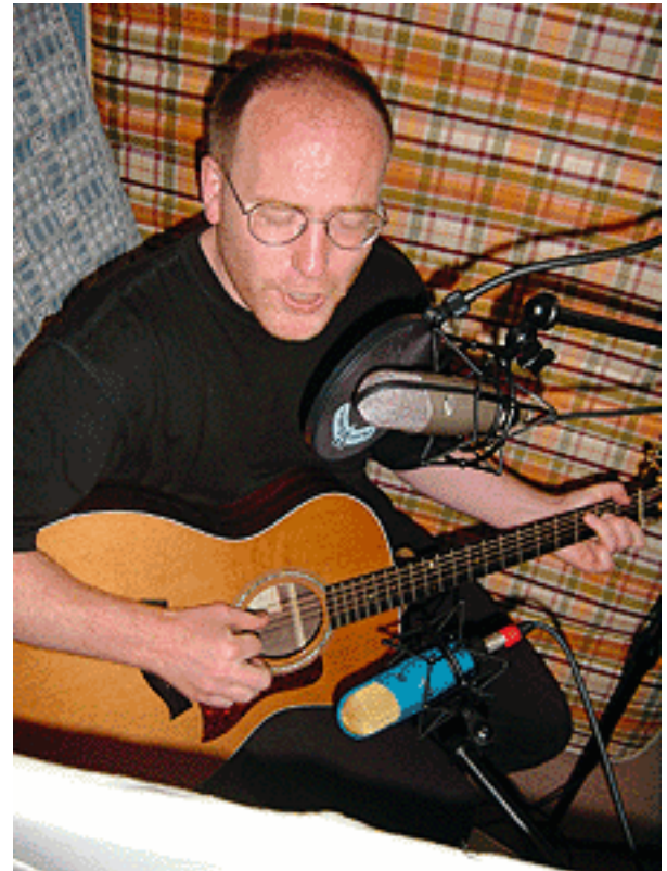
An improved setup using the two microphones in figure-of-eight mode.
