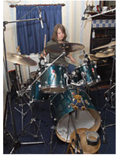
A pair of condenser mics used as stereo overheads really helped give a more professional sound. Positioning them a little further back gave a less cymbal-heavy balance, which meant that only a little of the each close mic was required to focus the sound of the drums.
