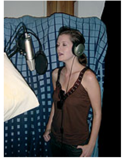
Getting a good vocal sound required draping a duvet behind the singer and taping a pillow to the mic stand — this reduced the level of room sound reaching the mic, resulting in a less coloured and more usable sound.
