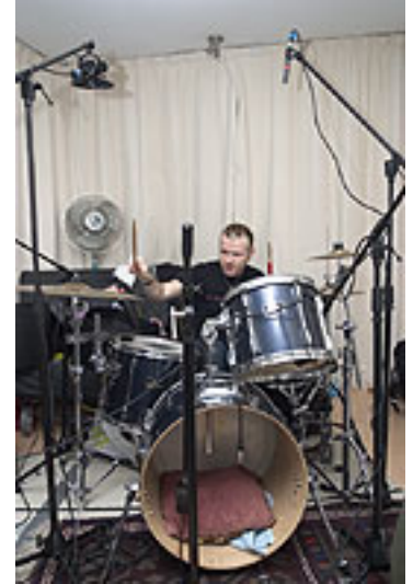
Although a stereo pair of overhead mics was not available, an unmatched pair (Audio-Technica AT4033 & AKG SE300) still gave a very usable sound once the levels were matched.
