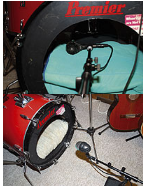
Peter's original kick mic positioning several inches outside the body of the drum didn't give nearly as much definition to the recorded sound as miking close to the batter head inside the drum.
