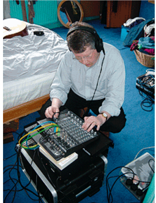
Hugh Robjohns auditions recordings through Steve's Mackie 1202 VLZpro mixer — although Steve's VS1680 recorder has a headphone output, better results were achieved by monitoring the main outputs through the external mixer.
