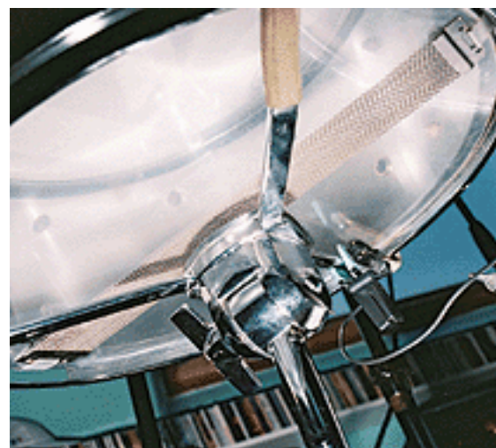
The snare was miked with an SM57 above and an AKG C418 miniature clip-on mic below.
