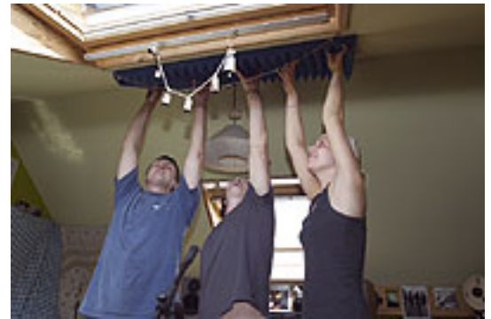
Tony and B helped Paul temporarily place some acoustic foam on the ceiling to see whether ceiling reflections were compromising the monitoring sound.
