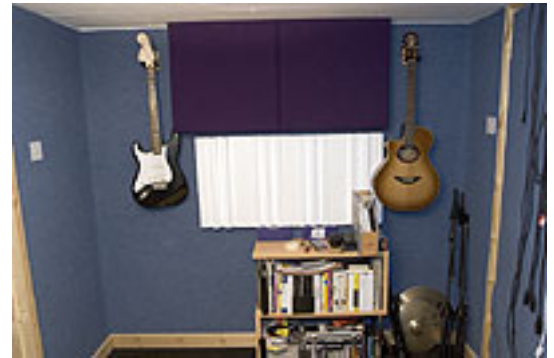
Another foam panel was placed on the rear wall of the studio, along with a polystyrene diffuser designed to combat the high-frequency absorption of the carpeted studio walls.
