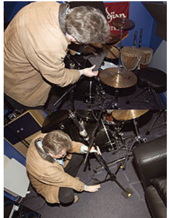
Foam was fitted around the snare mic to reduce spill, and more foam was used to isolate some of the mic stands from mechanical vibrations, as none of the mics used had proper shockmounts.
