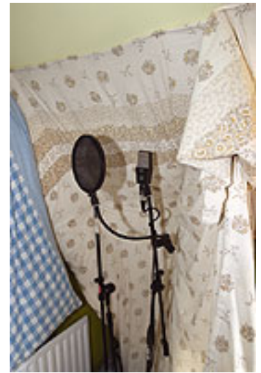
This is the vocal recording setup Tony had been using. Paul & Hugh recommended that he face the mic back into the padded corner, rather than into the room, in order to reduce the amount of room sound captured.
