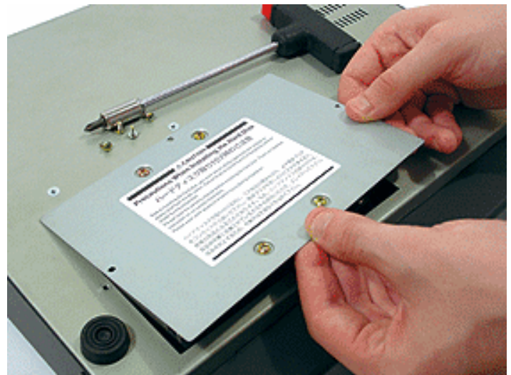
Removing the hard drive access plate of the Fostex VF16 located the loose screws responsible for a mysterious rattling noise during recording.
