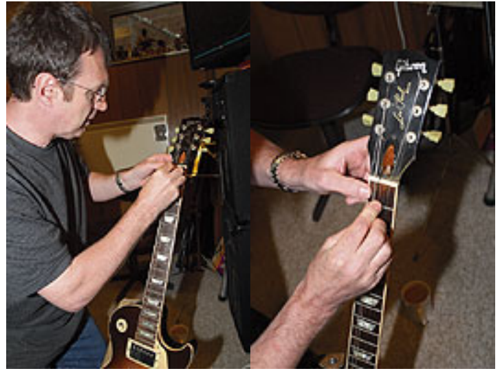
The action of Peter's Gibson Les Paul Standard was set too high, so Paul used an old junior hacksaw blade to deepen the nut slots slightly, but suggested that Peter also have the instrument set up professionally as soon as possible.
